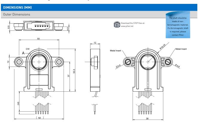
Sensor shown above is the 17mm version with the rotor at zero position. The sensor is delivered in a random position. Wires: 0.35mm² TXL SAE J1128
